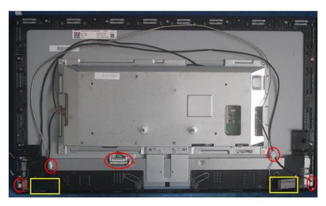
S5.Remove the screws to separate the panel and the Middle Frame, DECO BEZEL and the LED board.
