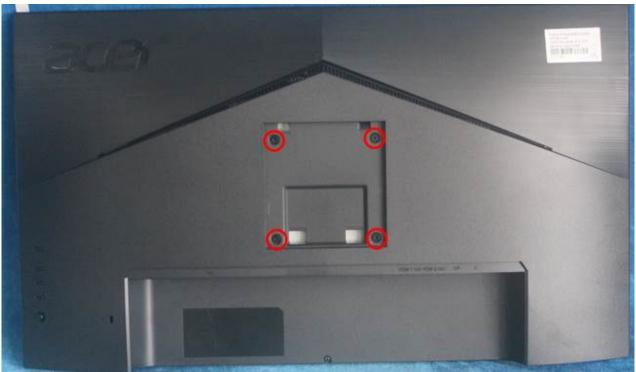
S2.Remove the rear cover. Use a tool (like picture using) to open all latches. (Be careful the position of the key board.)
